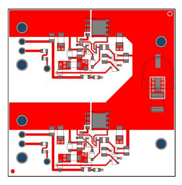
Figure 5: PI2007-EVAL1 layout top layer. Scale 2.0:1
