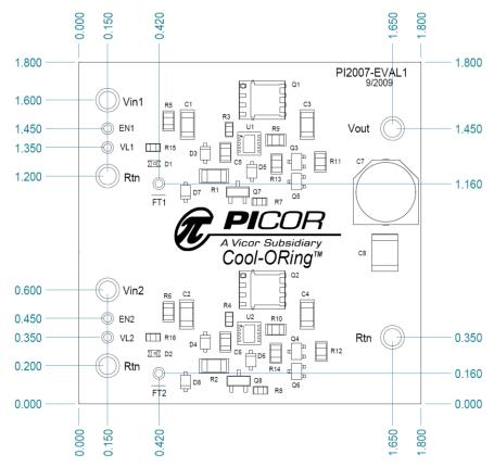
Figure 7: PI2007-EVA1 evaluation board mechanical drawing.
