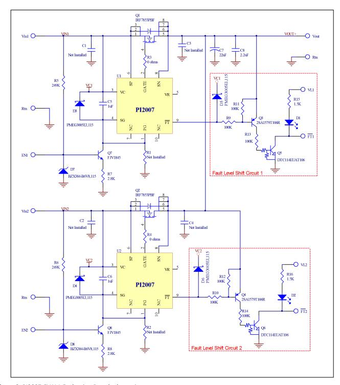
Figure 2: PI2007-EVAL1 Evaluation Board schematic.
