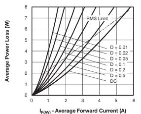
Fig. 5 - Forward Power Loss Characteristics
